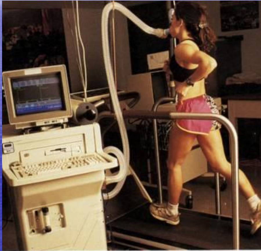
Figure 5.11 The equipment used to measure the respiratory exchange of oxygen and carbon dioxide.
